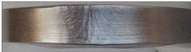
Face (Non-Crack )    Root (Non-Crack )
